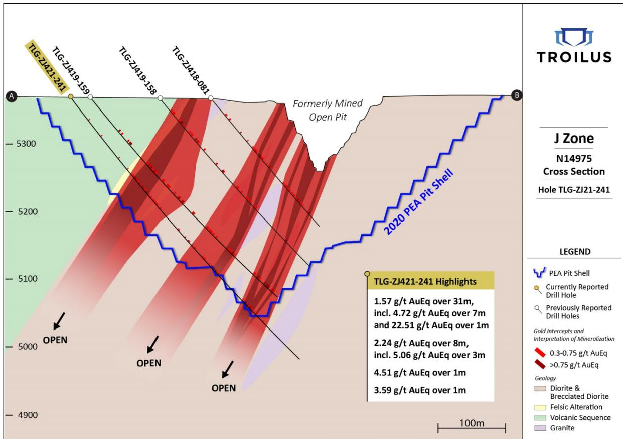
Figure 2: Section N14975; View of drill hole TLG-ZJ21-241
