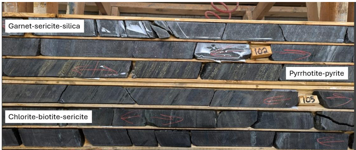
Figure 2. Zonation in alteration centered on the mineralized zone (WR-24-003: 1.66 g/t AuEq over 20m, incl. 3.10 g/t AuEq over 8m)
