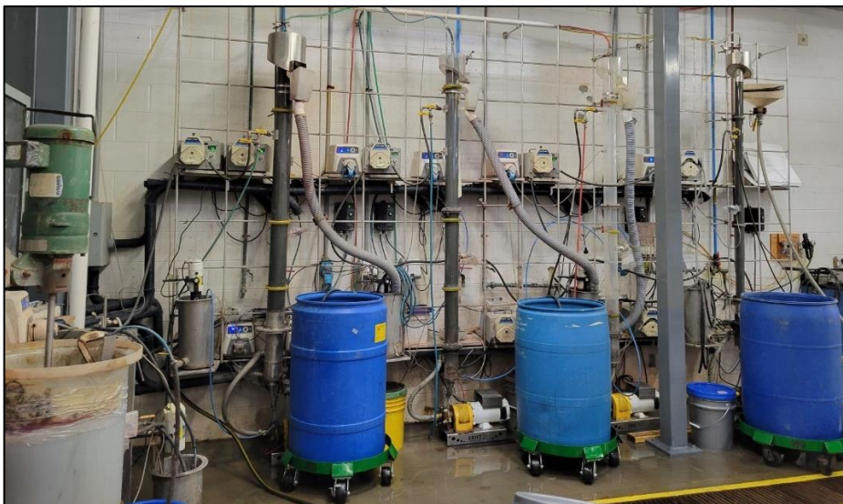
Figure 13-13 Eriez Pilot Plant 4-inch 1 st Cleaner, 3-inch 2 nd Cleaner and 2-inch 3 rd Cleaner Columns
