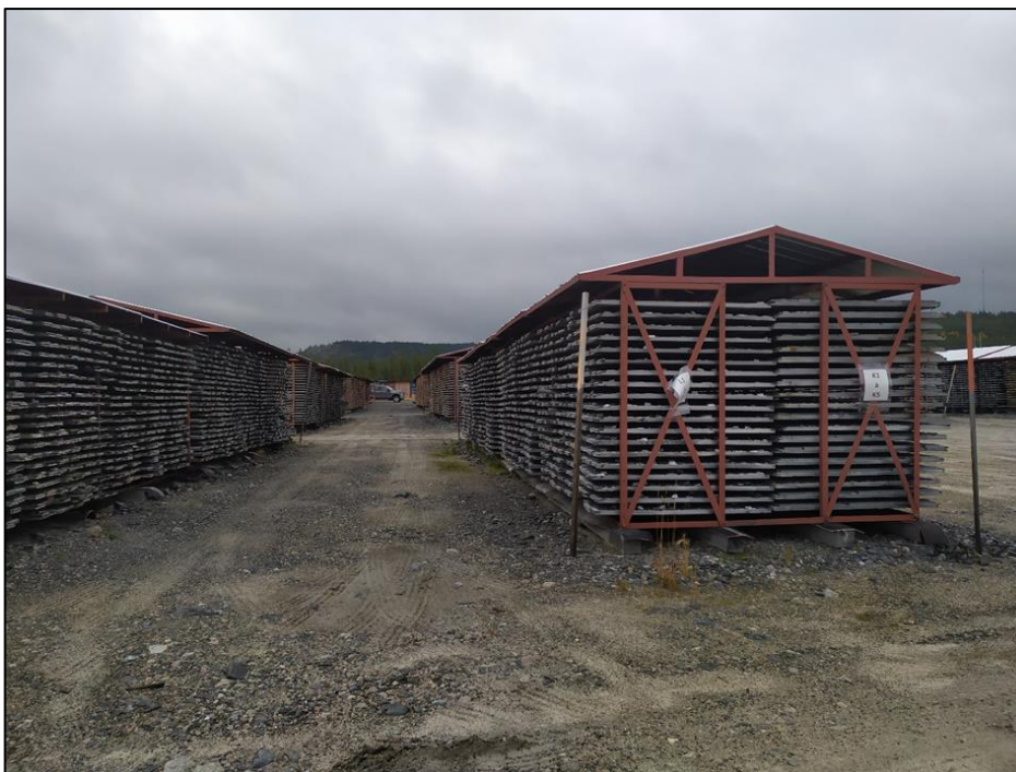
Figure 12-4: Core Storage Area; Core Racks
