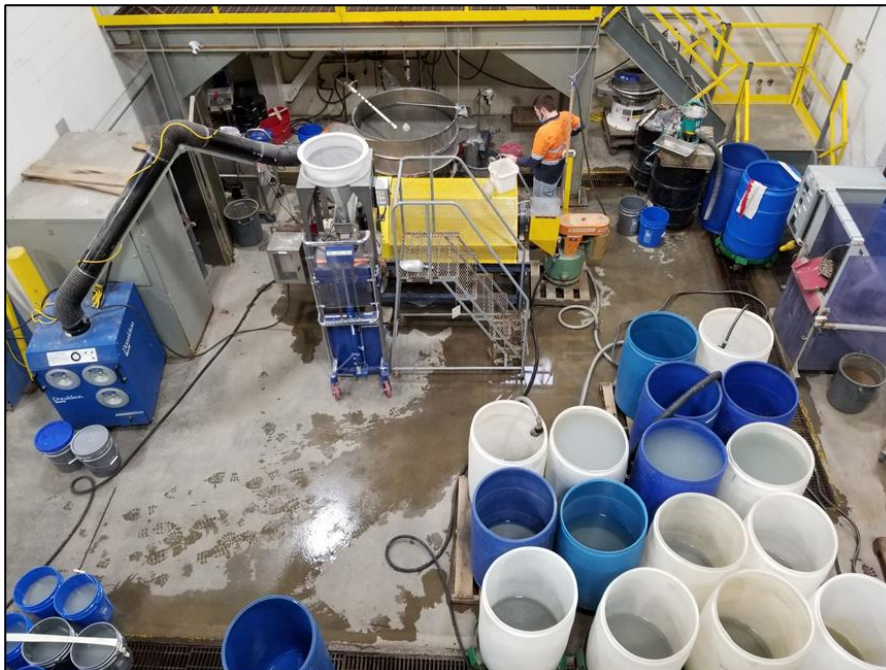
Figure 13-11 Eriez Pilot Plant Ball Mill and Gravity Recovery Circuit
