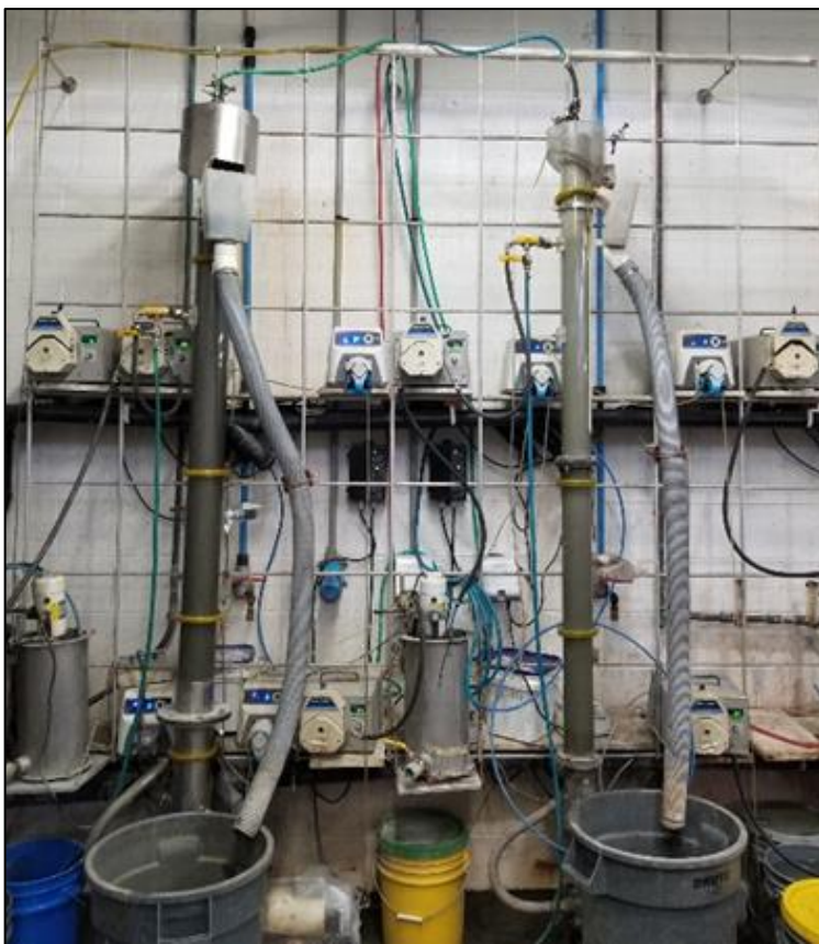
Figure 13-12 Eriez Pilot Plant 4-inch Rougher Column and 3-inch Scavenger Column
