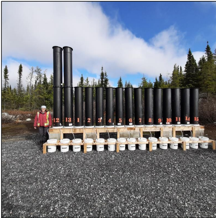
Figure 20-7: Field Columns Built on Site
